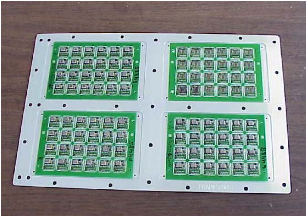
Carrier pallet for array of ASIC TCXOs. The array will be separated into individual TCXOs later in the process. The carrier pallet will nest the individual TCXOs also.
