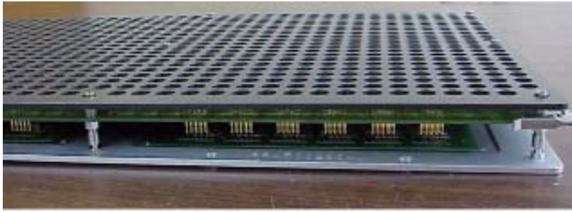
ASIC Test Board for with support pallet. One of many options to hold DUTs.
