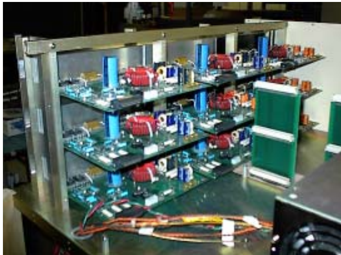
Chamber top with the 9 power supplies mounted (the control boards are not present). The triple board vertical back plane assembly from the chamber innards is visible
